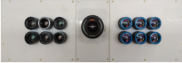
Figure 1: Broad band multi-aperture snapshot camera in the IR (0.4-14 \mu\text{m} ). Left: MWIR module, centre Visible and NIR, right LWIR.
